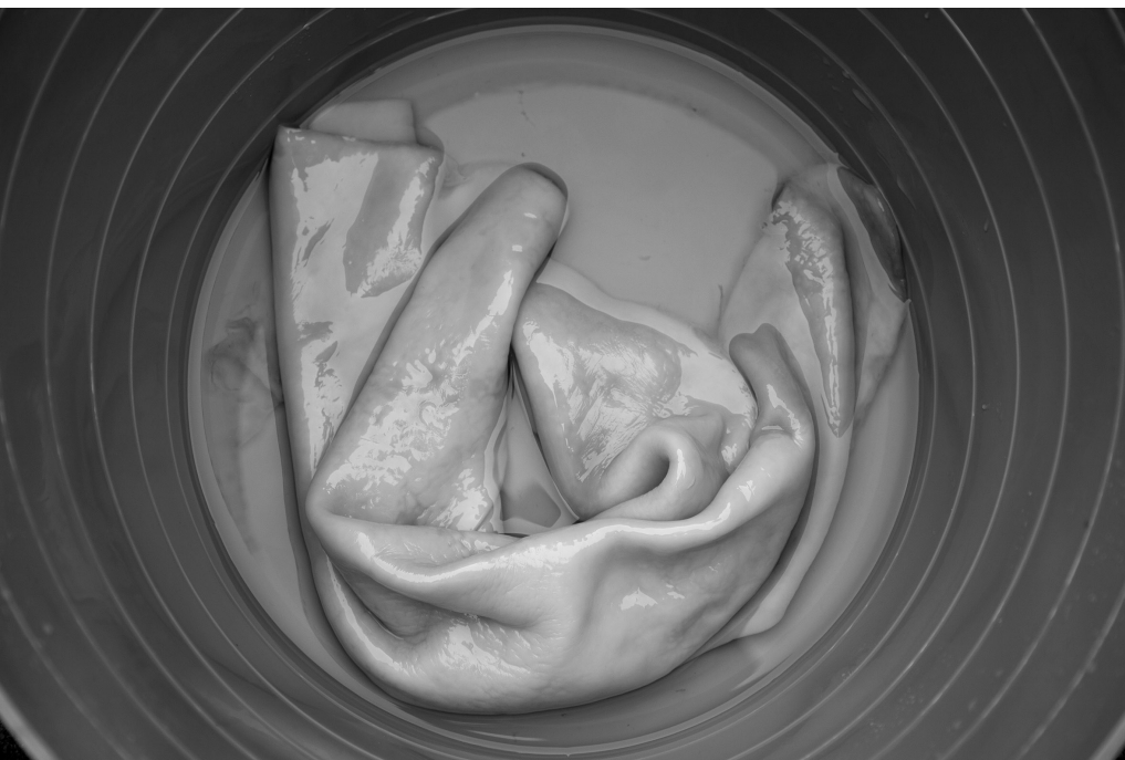
Figure 9. Bacterial cellulose in the process of being washed. Image by Ingrid Rhule.
